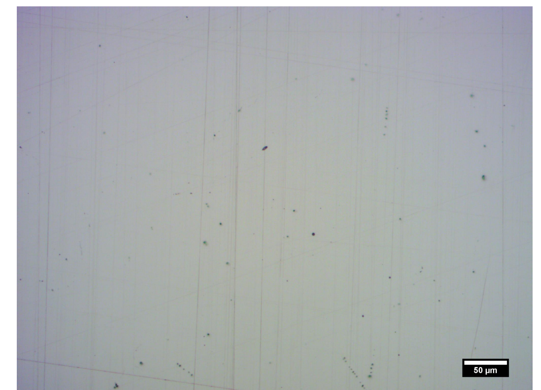
Figure 9: Optical image of a crack-free, DMLS-fabricated Alloy 230 sample from DOE 2, using 30 \mu m layer thickness.
